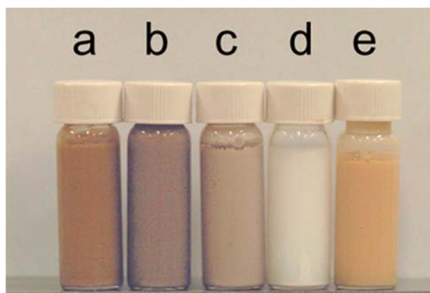
Fig. 1 Photographic image of surface modified P25 nanoparticles and the nanoconjugates of TiO 2 @Ag. (a) 5 g/L AT050 functionalized with DHBPA; (b) 5 g/L AT050; (c) 5 g/L AT025; (d) 5 g/L bare P25; and (e) 5 g/L bare P25 functionalized by using DHBPA
